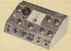
The Polarography Module and the capabilities of the Heath Polarography Laboratory are described on page 100.
