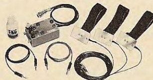
Bioelectric. IMPScope shows bioelectric phenomena in plants (175 mv action potential of Nitella internode).
